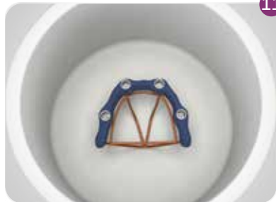
Castable ring with waxed framework.
